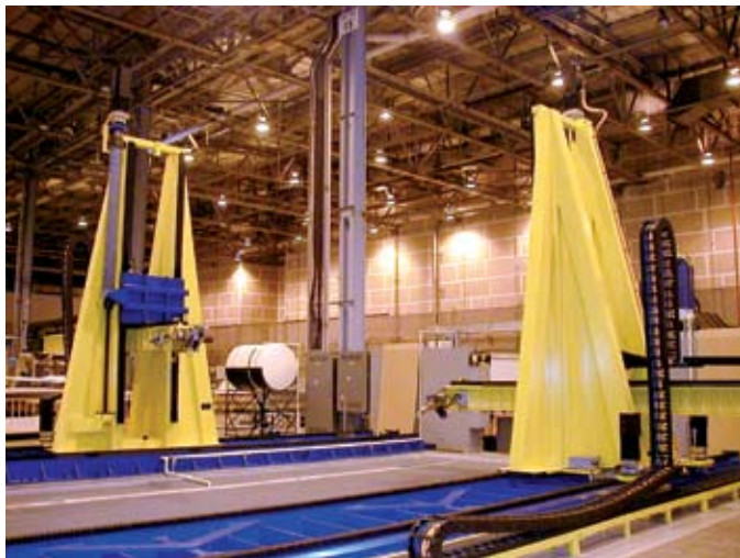
The National Center for Advanced Manufacturing's Non-Destructive Evaluation System employs a twin 5-axis traveling column configuration and multiple inspection system capability. (LMSSC-MO)
