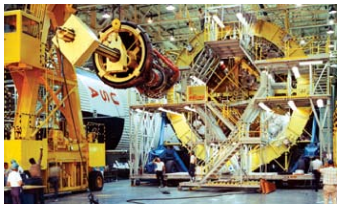
Engineers at NASA's Michoud Assembly Facility install an F-1 engine on the Saturn V S-1C first stage. The S-1C first stage included five F-1 engines and powered the Saturn V rocket through the first 37.9 miles of launch. (NASA/MSFC)
