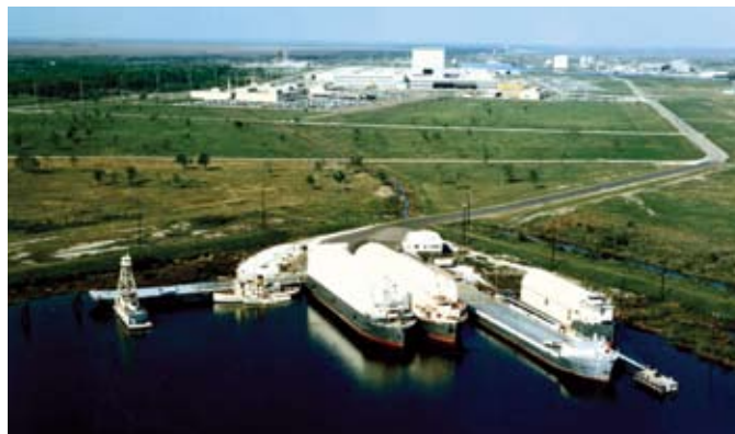
An aerial view of the NASA dock at Michoud Assembly Facility with four barges – from left, the Paleamon, Promise, Poseidon and Orion. The barges ferried the Saturn IB and Saturn V upper stages between Michoud; NASA's Marshall Space Center in Huntsville, Ala.; Stennis Space Center near Bay St. Louis, Miss.; and Kennedy Space Center, Fla. (NASA/MSFC)
