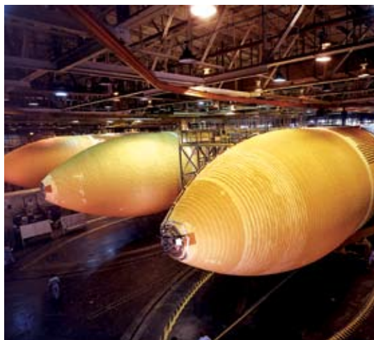
The final assembly phase of space shuttle lightweight external tanks 5, 6 and 7 is under way at Michoud. Each giant cylinder, taller than a 15-story building, is 154 feet tall and 27.5 feet in diameter. The external tank is the largest single piece of the shuttle system. (NASA/MSFC)
